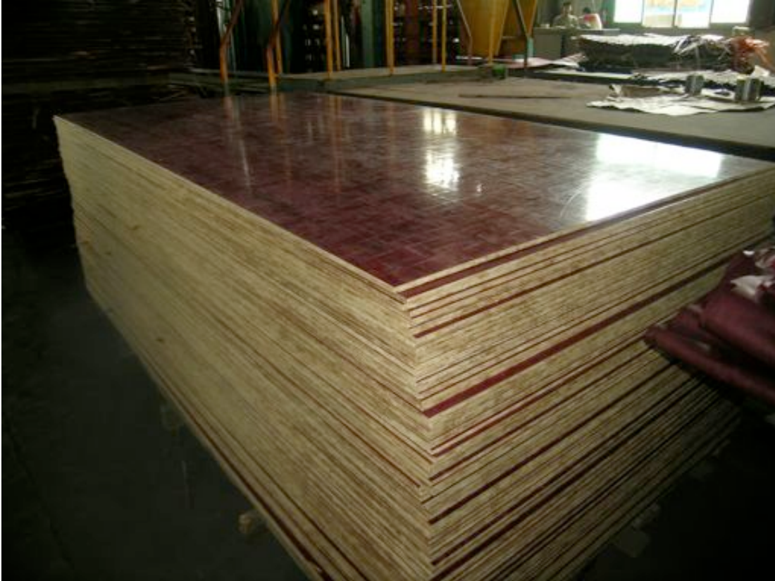
Figure 7-4. Bamboo boards used in foundations (Photo: Badrkhan 2005).
