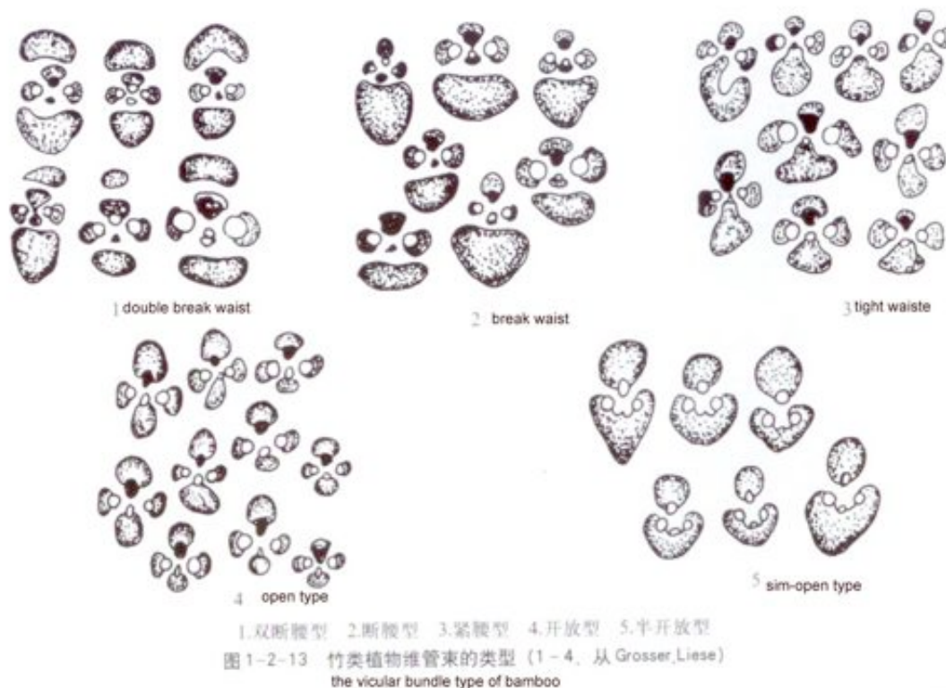
Figure 2-7. Vascular bundle types of bamboo. 1- Double break waist and 2- Break waist (vascular bundles in sympodial bamboo), 3- Tight waist (amphipodial mixed bamboo vascular bundle), 4- Open type and 5- Sim open type (Monopodial bamboo vascular bundles) (The Chinese text book in Chinese).
